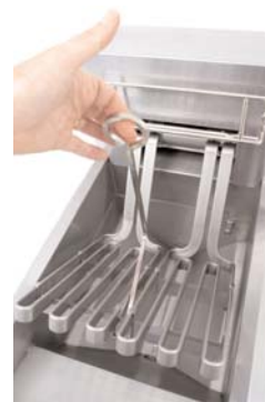
Combines swing-up elements with controlled burn-off cleaning (RE14 illustrated). Lift handle not available on 22 kW split pot element assembly.
