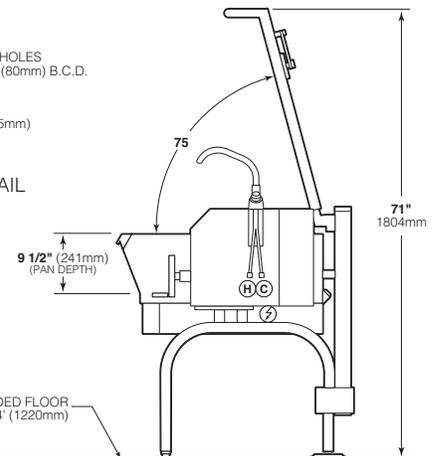
RECOMMENDED FLOOR SLOPE 1" (26mm) IN 4' (1220mm)
