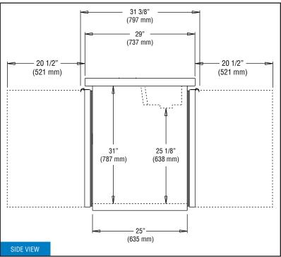
IMPORTANT NOTE: Models are completely front breathing and take in and exhaust air through the front grill. For proper operation, the area in front and back of the cabinet must not be obstructed in any way. A clearance of 3" on the sides is recommended.
