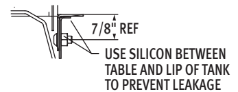
Sectional View Showing Table Connections
