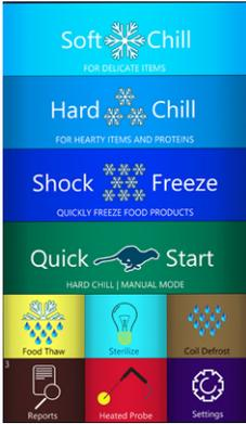
**Soft Chilling:** The air temperature is held in the range of 28°F to 35°F, ideal for delicate food items. The chilling cycle is completed when the food core temperature reaches 38°F.
