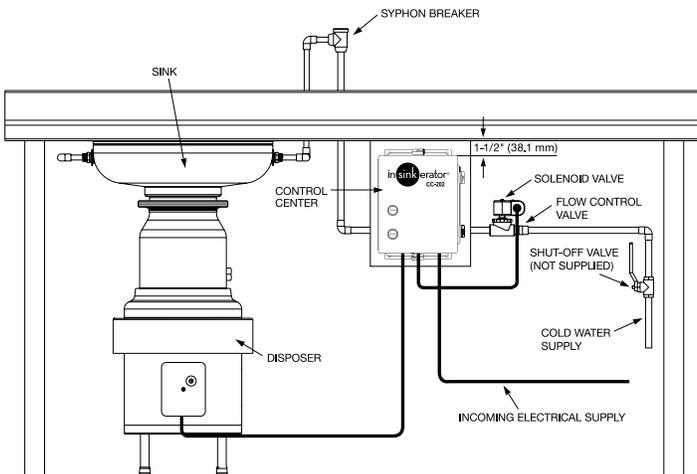
**NOTE:** The CC-202 control center should be mounted 1-1/2" (38.1 mm) back from the front surface of the table.
