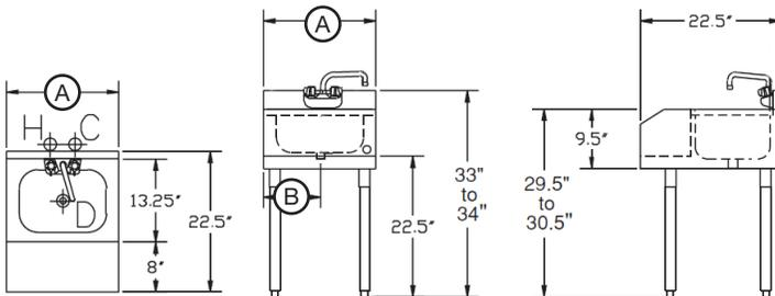
**Mechanical Requirements:** 1/2" IPS hot and cold water. 1-1/2" IPS drain connection.
