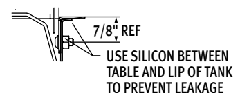
Sectional View Showing Table Connections
