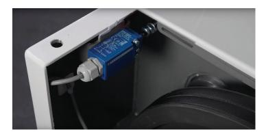
The safety limit switch is located inside the machine to prevent possible tampering.
