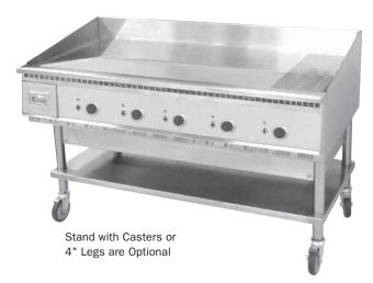
The Keating MIRACLEAN® Griddle is designed to provide maximum performance with many benefits to the operator. The mirror surface is achieved in a special eight step process. Insulated stainless steel electric elements are mounted every 12" to ensure performance and recovery allowing the operator to use zone cooking for different products.
