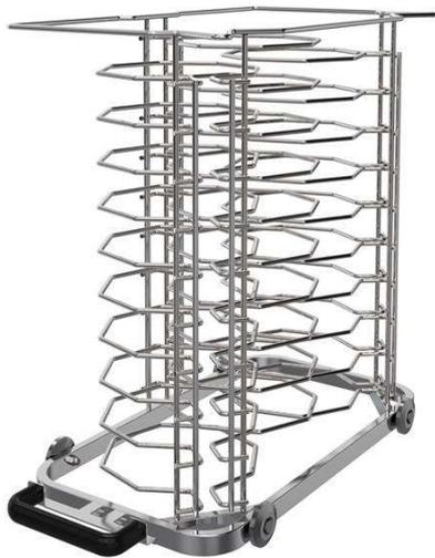
**922760 (TRBA92PL2021C)** Banquet trolley with rack holding 92 plates for 20 GN 2/1 oven and blast chiller freezer, 85mm pitch
