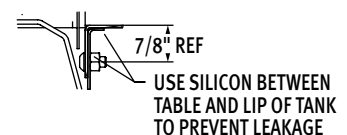
Sectional View Showing Table Connections
