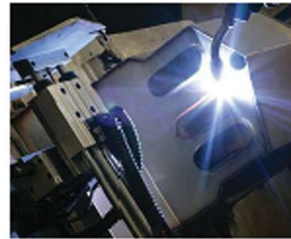
Robotic welding is precise, virtually eliminating leaks.
