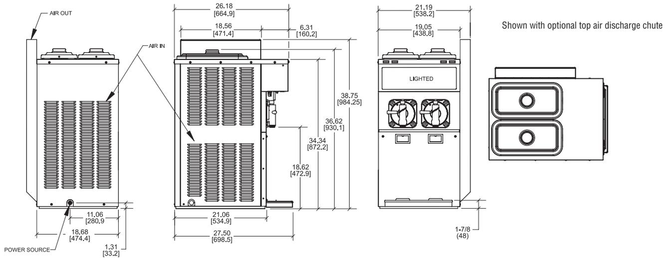
NOTE: FIGURES IN PARENTHESES INDICATE MILLIMETERS. / ALL DIMENSIONS PLUS OR MINUS 1/16 inch [1.5mm].
