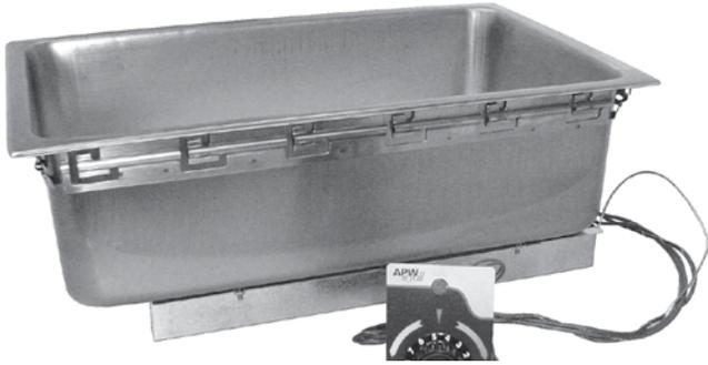
APW Wyott uninsulated drop-in hot food wells are supplied with a UL Listed approved electrical kit includes an electrical conduit, control box and bezel or a UL Registered kit with thermostatic controls, pilot light and a 36" capillary.
