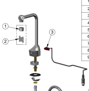
ITEM DESCRIPTION SALES NO. NO. VR 1.5 GPM Laminar Flow Device (Anti-Microbial) 1 B-0199-06-LF15A w/ VR Key 2 015425-45 Vandal Resistant Key 3 019174-45 Sensor Cable Asssembly Inlet Hose, Faucet, 1/2" NPSM-F x 1/4" NPSM-F 4 016297-45 5 ChekPoint Control Module w/ Filter Tee 019944-45 6 5EF-0002C AC Adapter - US Plug 7 5EF-0005 Supply Hose, 9/16-24 Female x 1/2" NPSM 8 002534-25 Close Nipple, 1/2" NPT 9 **EC-FILTER** Replacement Filter
