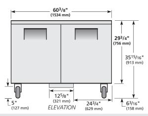
METRIC DIMENSIONS ROUNDED UP TO THE NEAREST WHOLE MILLIMETER
