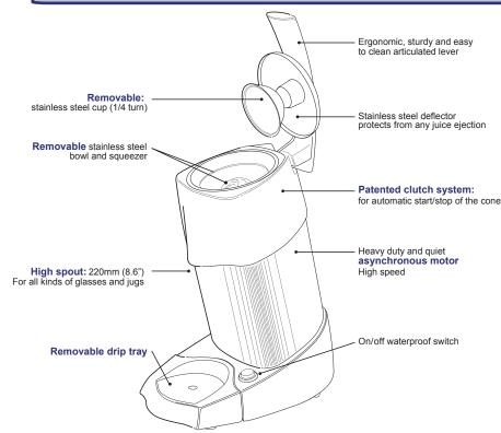
The lever juicer evolution #70 is the ideal product to make fresh juices from lime, lemon, orange and grapefruit. Thanks to its powerful motor and its high output (501/h) is adapted for intensive use.
