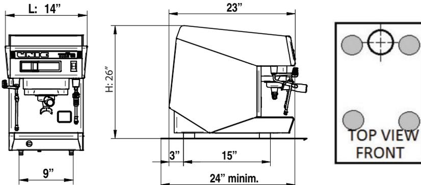
**PLEASE NOTE:** There are 3 inch leg extensions shipped with the machine, but not installed. Their use is optional, but highly recommended for ease of cleaning under the unit.
