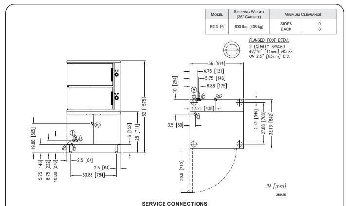
() – ELECTRICAL CONNECTION: Field wiring electrical connection to be as specified on data plate.
