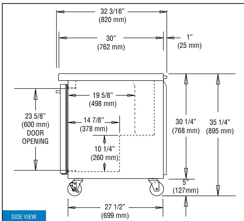
**IMPORTANT NOTE:** If the cabinet is located directly against a wall, a minimum clearance of 3" is required on sides, front and rear.
