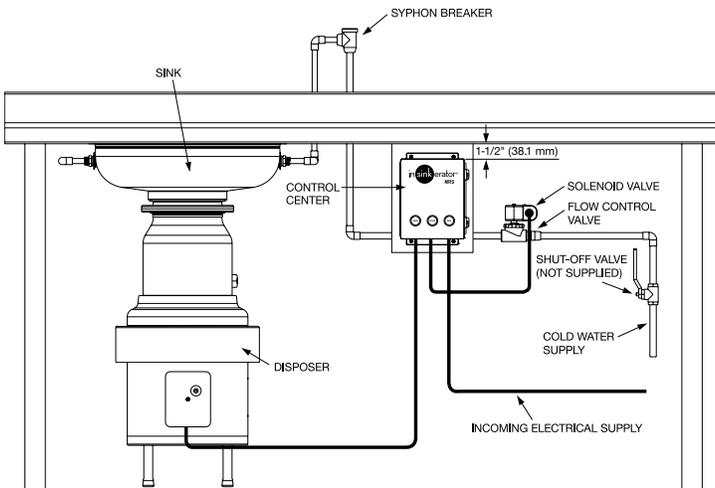
**NOTE:** The MRS control center should be mounted 1-1/2" (38.1 mm) back from the front surface of the table.
