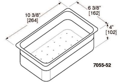
**Wet Waste Box - With Drain Tube**
