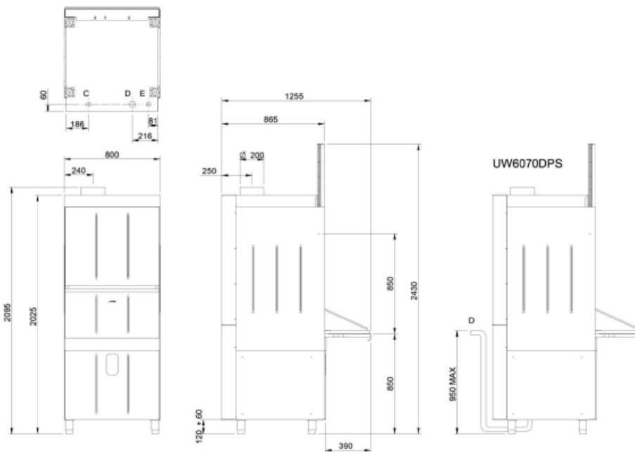
D = SCARICO 1/2", VIDANGE 1/2", DRAIN 1/2", ABFLUSS 1/2", DESAGÜE 1/2", СИДБ 1/2"
