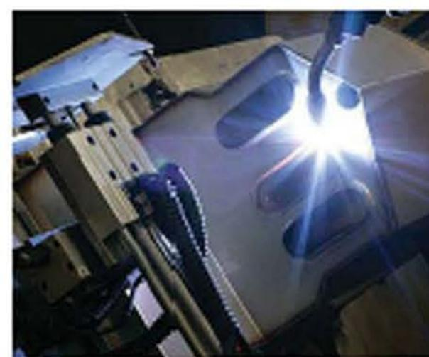
Robotic welding is precise, virtually eliminating leaks.
