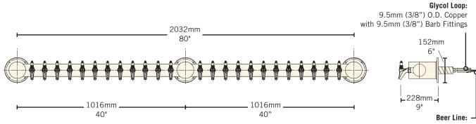
6.4mm (1/4") O.D. Stainless Steel with 6.4mm - 9.5mm (1/4" - 3/8") Tapered Barb Fitting
