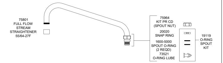
PRODUCT SPECIFICATIONS: SWING SPOUT WITH OR WITHOUT FULL FLOW LAMINAR STREAM STRAIGHTENER, FITS FISHER SWIVEL OUTLETS
