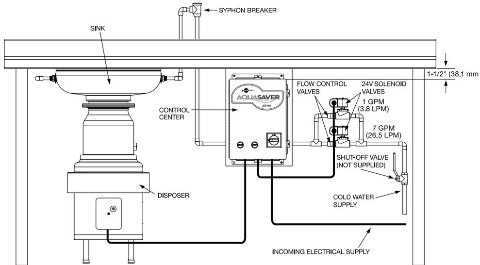
NOTE: The AquaSaver® control center should be mounted 1-1/2" (38.1 mm) back from the front surface of the table.
